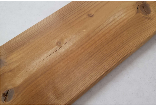
Small surface cracks are allowed.
