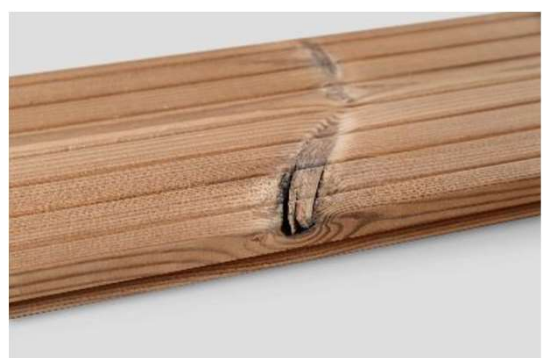
Small dry (loose) knots on the edge of the board are allowed.
