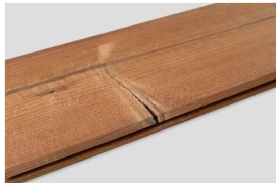
Individual splits of (live) knots are allowed. In spruce, the cross checks of the knots belong to the general appearance.
